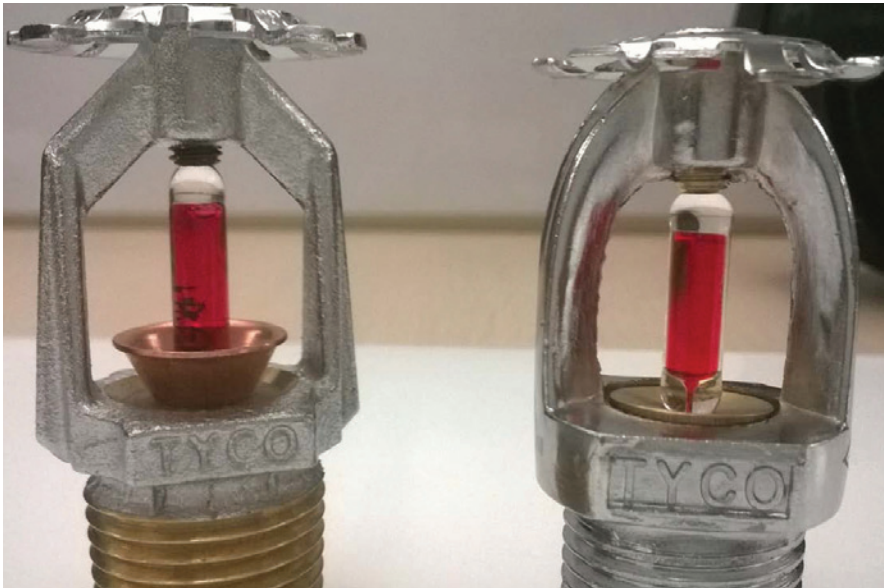
Profile view of an authentic Tyco TY3251 sprinkler (left) and the sprinkler identified as counterfeit (right).
