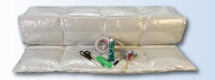
Ever Green CHW — Each kit contains one 4 ft. x 8ft. modularized 2" insulation blanket with a zero-perm vapor retarder on both sides, a 75 ft. roll of 4" wide zero-perm pressure sensitive tape, a 3 fluid ounce tube of silicone caulk and a utility knife.
