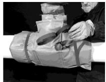
9. For a gate valve, continue installing the third blanket around the valve body. It may help to snip several inches into the Cut 'n Wrap blanket seams to get a
