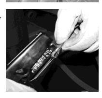
3. Cut the required blanket pieces from the roll of Cut 'n Wrap. **Note:** Insulation for a **flange** should consist of one blanket piece of the
