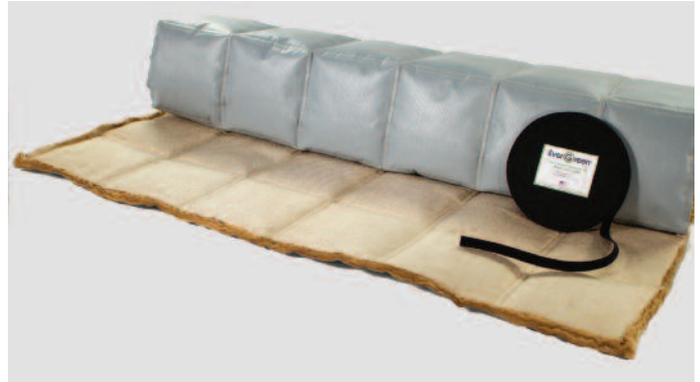
*Ever Green® ET Cut 'n Wrap is an engineered insulation composite with a fiberglass inner core, a high-performance-polymer-coated woven glass fiber fabric outer layer, and a woven glass inner (challenge) layer.*
