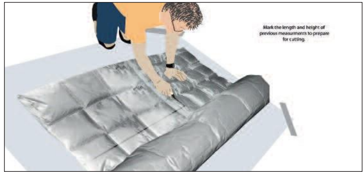
Figure 3 — Marking blanket to indicate cuts
