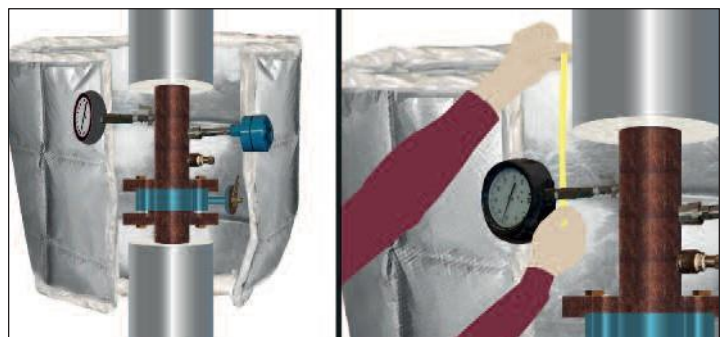
Figure 6a, 6b — Measuring and marking the blanket for one of the penetrations
