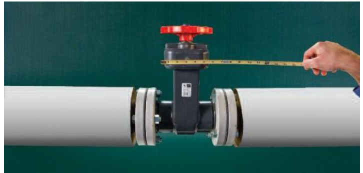
Figure 1 — Measure pipe length and circumference (a & b)
