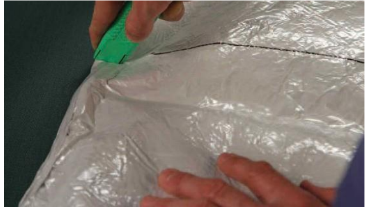
Figure 4 — Cuts should be made with blanket laying on a flat cutting surface
