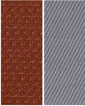
Silicone can be applied to either one or both sides of AMI-TUF® for added moisture and oil resistance.
