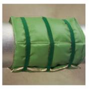
AMI's new Ever Green® Cut 'n Wrap™ insulation kits\* are ready-to-use, removable and re-usable insulated covers for steam and hot water distribution piping valves, flanges, fittings and other hard-to-get to components. Each kit comes with a 32 square foot modularized insulation blanket and one 75 foot roll of double sided hook and loop fastener.
