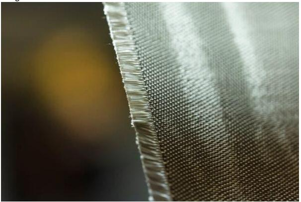
Fiberglass fabric before it is processed in a vertical oven, where it will be heated at 1,300 degrees Fahrenheit to caramelize so it won't smoke when reaching high temperatures. Credit... Yoon Byun for The New York Times
